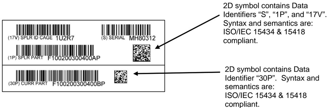
NOTE: CEA 802 protocol and UII Construct #2 using Data Identifiers encoded in Code 128 and Data Matrix ECC 200 symbols. It is an example of how the mark may be changed after the item is altered. The current PIN could be added to the mark or the current PIN could be replaced if it was part of the original mark (compare Figure 4.a with 4.b). The original PIN is retained and the current PIN is added or changed as shown in the bottom section of the label.
