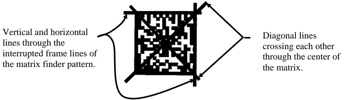
**FIGURE 14. Obliteration of a Data Matrix symbol.**
