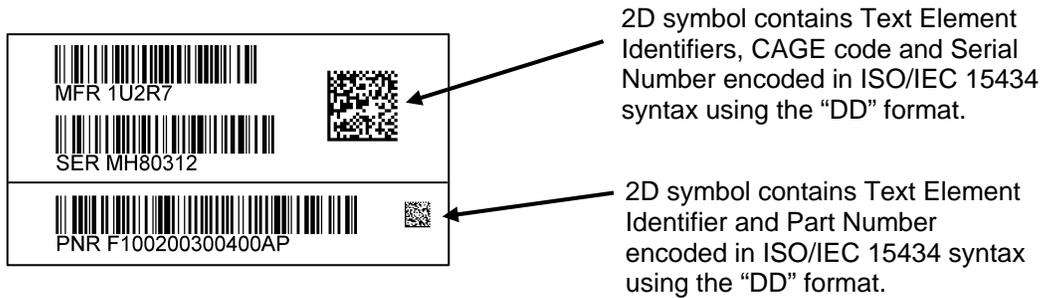
NOTE: SPEC2000 protocol and UII Construct #1 using Text Element Identifiers (TEI) encoded in Code 128 and Data Matrix ECC 200 symbols. The available TEIs listed in ATA SPEC2000 CSDD permit the use of UII Construct #1 for an item UID. The UII is established by the enterprise's identification and a serial number unique within that enterprise identifier. The current part number is shown on a separate label as per the ATA protocol.
